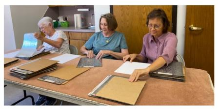
Janet Jamison, Marie Vavra and Corene Cline insert the numbered pages into zinc plates with braille indented on both sides of plates. The plates are then fed through a press.
